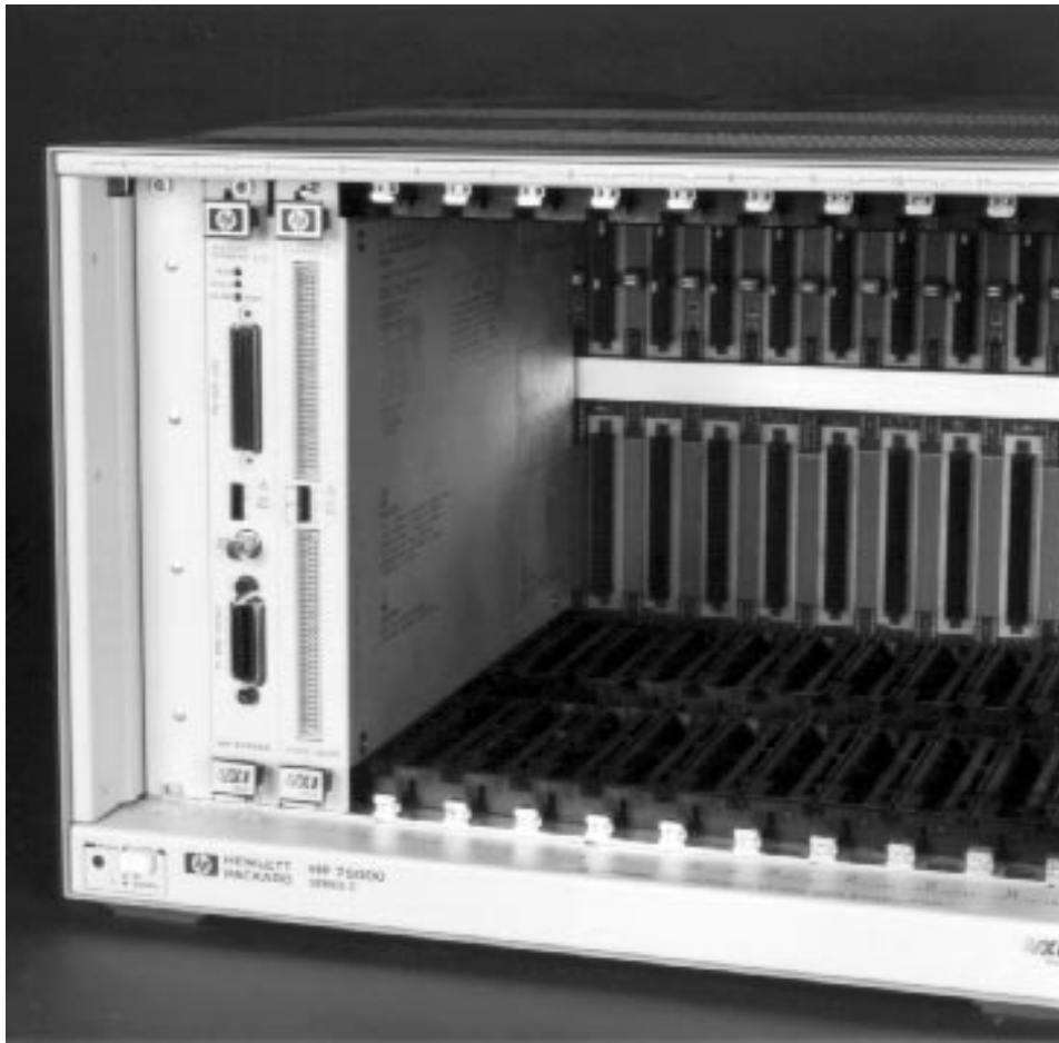
Fig. 1. The HP HD2000 data acquisition system showing the HP E1413 and HP E1414 modules.
