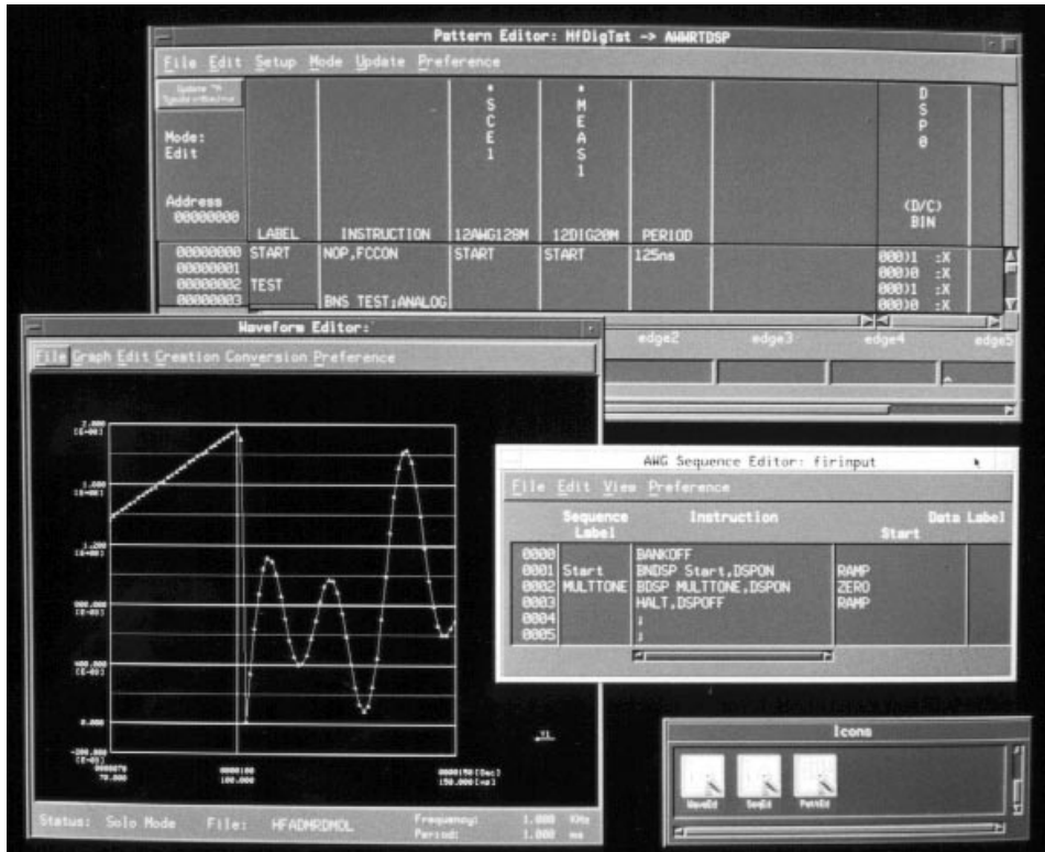
Fig. 3. Synchronous waveform switching. The highlighted window is an editor for programming waveform generation. The instruction BNDSP Start,DSPON switches data to the DAC. The waveform is displayed in the waveform editor window and shows the switching between the ramp from the waveform memory and the multitone wave from the DSP. The upper window is a pattern editor for programming a test sequence, the start and stop of the synchronous trigger, and digital patterns and formats. START in the SCE 1 column starts the arbitrary waveform generator sequencer and the DSP.
